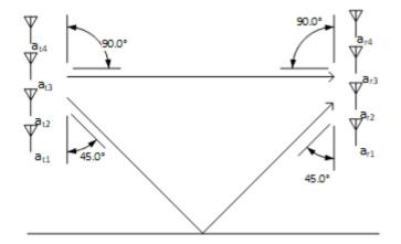
Figure 1: Arbitrary room with two antenna arrays. Between the arrays a direct path is present as well as a path along a reflector.
