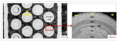
Figure 3: TEM top view of gate-all-around 'macaroni' FETs. The channel is now on the inside of the tube while the charge is stored inside the dielectric layers (note the atoms!). Source: Chipworks.
