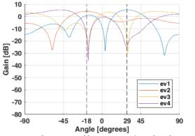
Figure 8: Angular sensitivity of the receiver array (rotated -30 degrees) for the simulation with a direct path and a reflection present.
