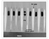
Figure 2: SEM cross section of a 16nm flash transistor string with a Control Gate and Floating Gate indicated. Adapted from TechInsights.
