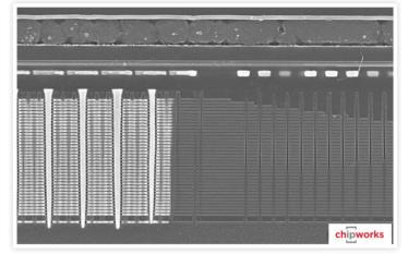
Figure 4: SEM cross section of a 32 layer 3D NAND CTF IC. Memory to the left, characteristic 'staircase' contacts to the right. Metal wiring on top. Source: Chipworks.
