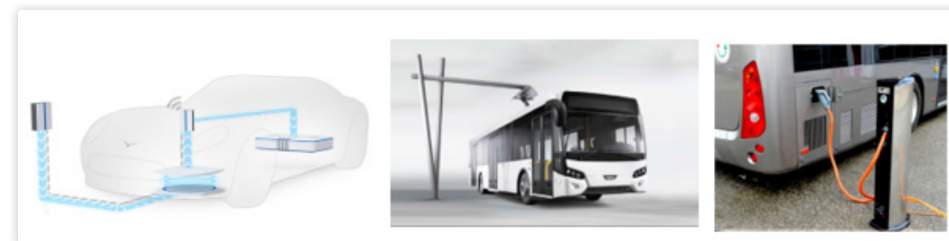
Figure 2: Charging methodology: inductive / pantograph / power plug
